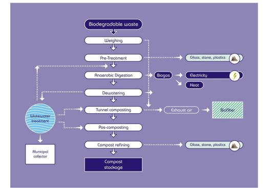
Figure 2. AD plant and process flow diagram.
